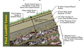
solid waste. The sides of the ET Cap are sloped enough to prevent ponding but not so steep as to encourage erosion. Water that does not infiltrate into the soil evaporates. The ET Cap soil contains nutrients that promote growth of native plants. Plants growing on the ET Cap absorb water in their root-system and then transpire the water back into the atmosphere. The combination of the evaporation and transpiration ("Evapo-
