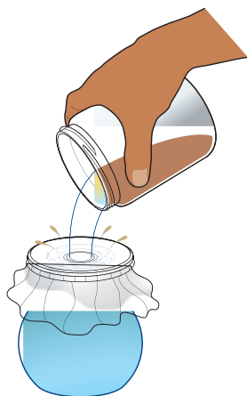
Figure 5.3. Straining water through a cloth
