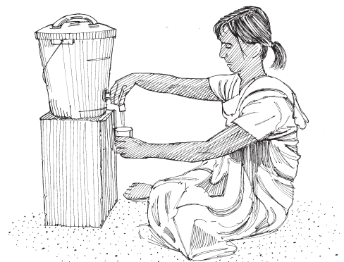
Figure 5.8. Tap fitted to a water bucket
