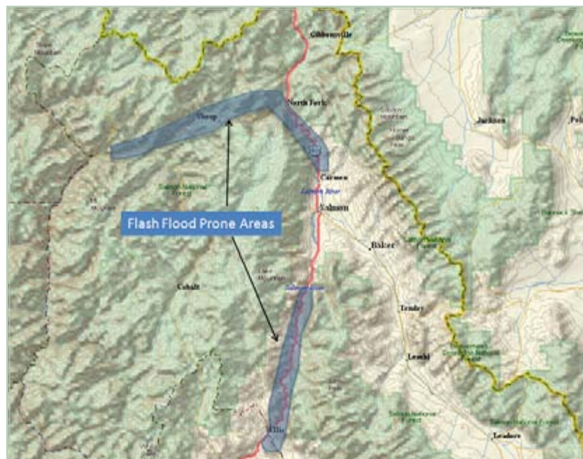
Figure 15: Flash flood prone area along Salmon River corridor in Lemhi County.
